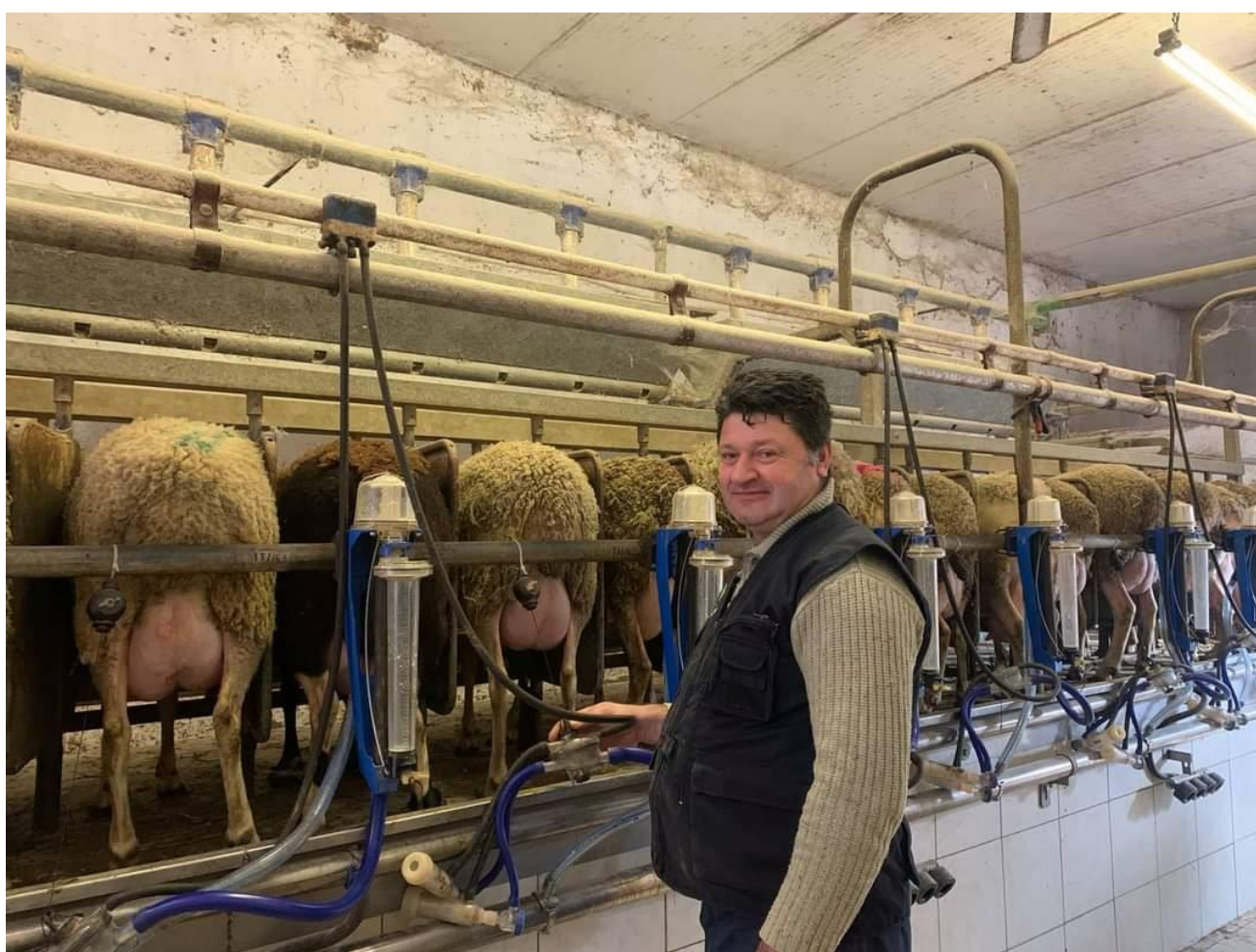
Individual analog volumetric milk meters installed at Iraklis' sheep & goat farm (© ELGO – DIMITRA)
